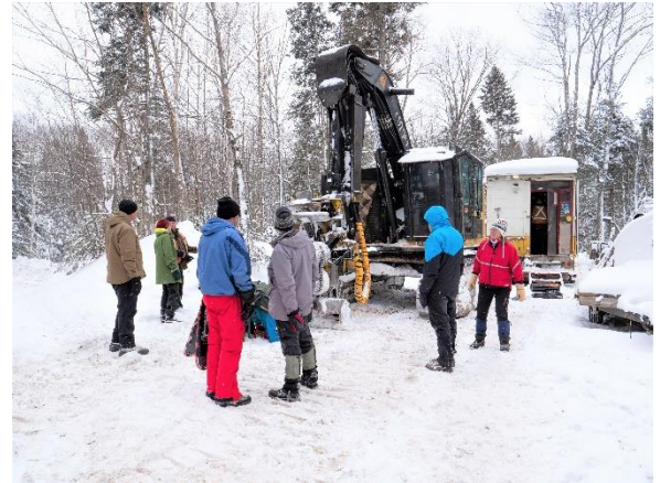
The Processor which limbs and cuts trees to length
