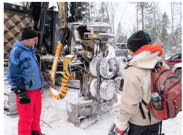
A closer look at the Processor's blades and saw
