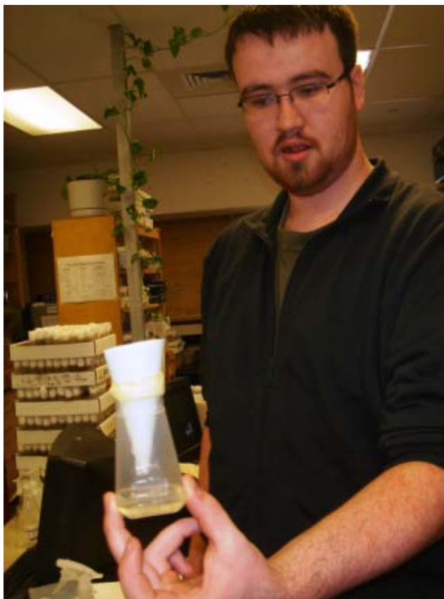
Student holding a simple trap used to catch fruit flies that escape. The Trap is a bottle with a funnel firmly taped to the mouth. The liquid is vinegar with a drop of dish detergent.
